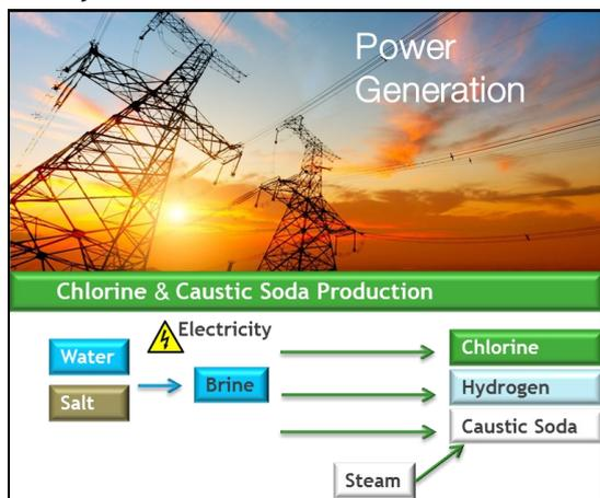
*An overview of the production of chlorine, caustic soda and hydrogen*
